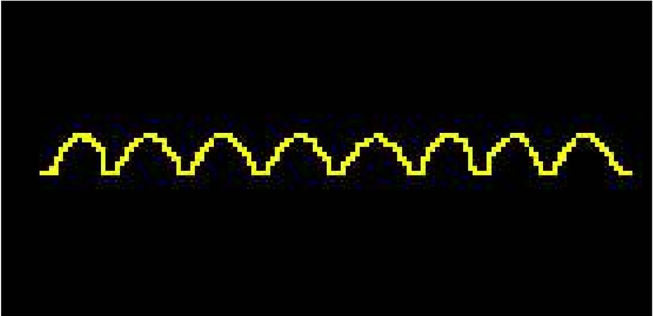
The most common failures are shorted or open diodes. Notice how large one of the diode patterns is in relation to the others this alternator needs work.
